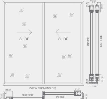
SL-55 has been exclusively designed to achieve highest strength and height. It is capable to withstand sash weight upto 220 kgs and height upto 3600 mm. Available with unique combination of manual and motorised integrated blinds.
